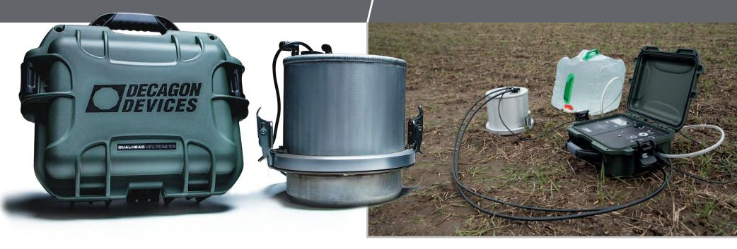
The new fully automated DualHead Infiltrometer measures (Kfs.), the ability of a porous medium to transmit water under saturated or near saturated conditions. The DualHead Infiltrometer uses the multiple head analysis approach to correct 3-dimensional flow without having to guess the Soil Sorptovoty (S) and the Soil Macroscopic Capillary Length ( $\alpha$ ).
